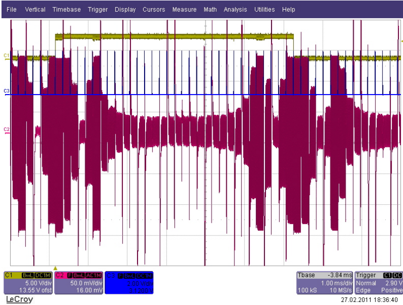
Figure D.1: Raw signal offset=4 “U-shape”. The yellow signal, used as trigger, corresponds to the injection switch digital command signal of active electrode 1. The red signal is measured directly after the differential instrument amplifier. The portion of the red signal comprised underneath the yellow signal at 5 V corresponds to a whole measurement frame period with injection between electrode 1 and 6. The blue signal is the synchronization signal, each time a pulse is generated the node fetch its next state in the scanning table. The red signal comprise between two blue signal pulse corresponds to a whole measurement windows.
